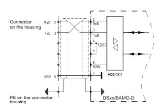
The serial interface is galvanically connected with the device zero (GND).
