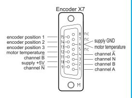
Use only motors with a Incremental (encoder) which have been approved by UNITEK (Appendix A).
