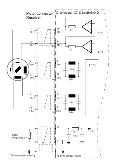
The resolver is an absolute measuring system for a motor revolution.
