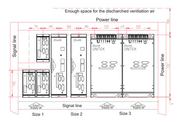
In order to achieve good EMC values, it is recommended to use bright, unpainted mounting plates. The bright surface of the device's rear panel ensure a good surface-to-surface contact.
