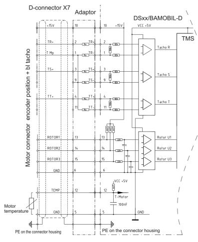
3 rotor position encoder signals (hall sensors) for the commutation; with or without a brushless tacho.
