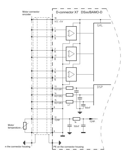
Incremental encoder (encoder) with 2 counter tracks and 1 zero track plus 3 rotor position tracks. Counter tracks with push-pull output.
