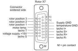
Only manufacturer-approved motors with incremental encoders and rotor encoders. Note motor specific connection sheet!
