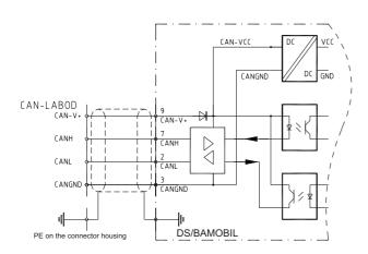
The interface is galvanically isolated from the device. The voltage is supplied via the bus cable.
